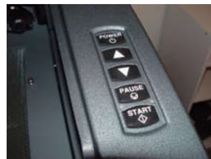
The VL-300 has only the most basic of controls on the cabinet because the system is primarily controlled through the software.
