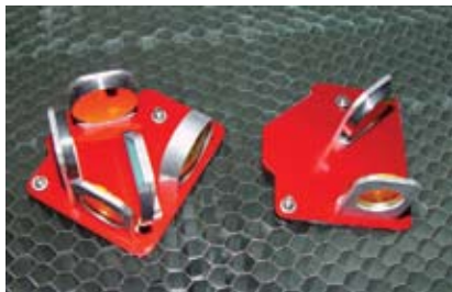
The lens on the right is the conventional lens and mirror assembly and the one on the left is the HPDFO lens.
